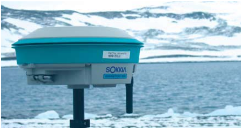
A Sokkia GSR2700 ISX GNSS receiver collects data despite the frosty Antarctic climate.
