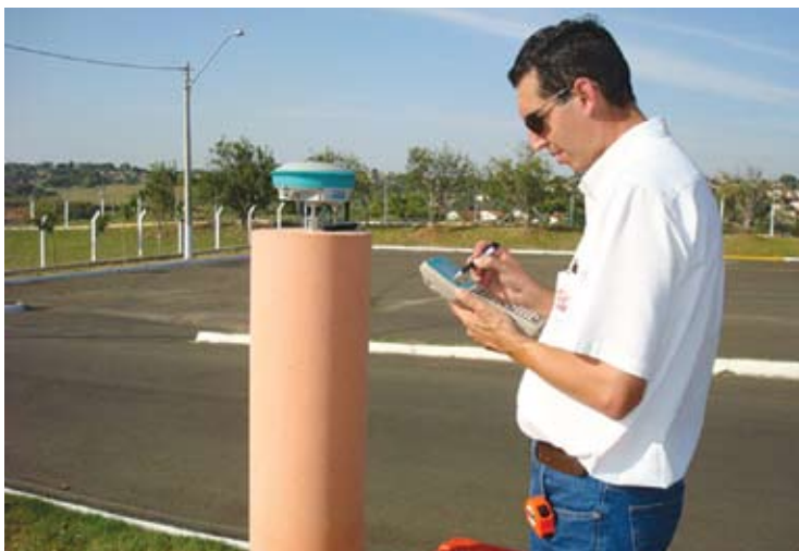
Jose Henrique Carvalho uses a GSR2700 ISX receiver to establish coordinates of the known geodetic monument SAT-93905.
